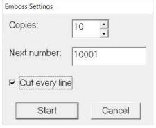
Number in the column of "Next number" automatically increases after print, according to printed Numbers.
