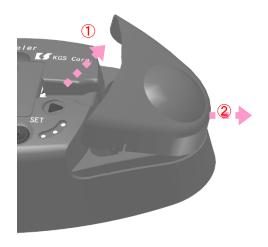
3. Remove a seal which fixes an edge of a braille tape on a roll.
