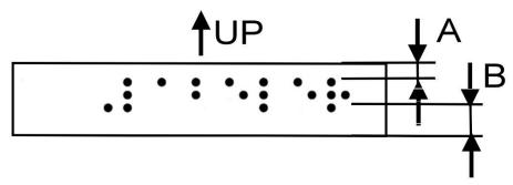
A black width of top and bottom has different one, after printed. Narrow one of blank width shows the upper part. (A<B)
