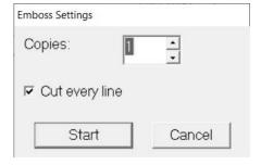
Check "Cut every line" in the check box, when cut a braille tape after printed dots by a scissors of BL-1000 LINK.
